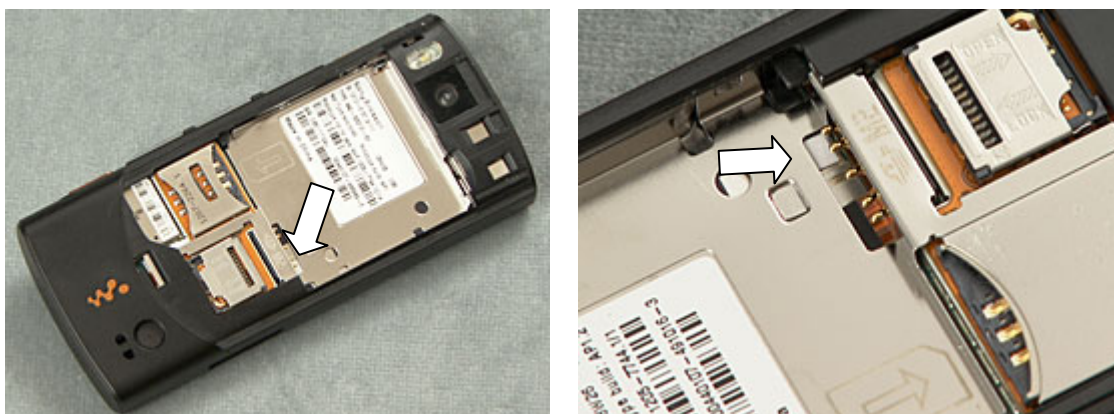
Location of the Liquid Intrusion Indicator. (Remove battery cover and battery)
